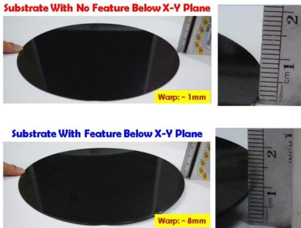
Fig. 12 Warpage comparison feature vs. no feature.
