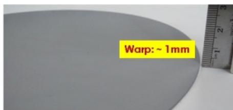
**Substrate With Feature Below X-Y Plane**
