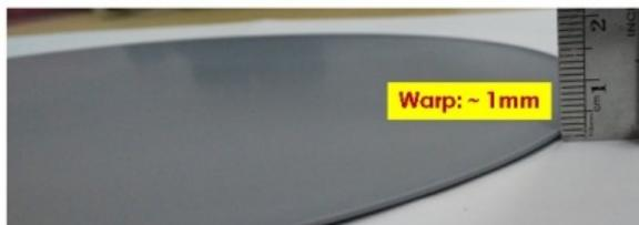
Fig. 13 Well design encapsulant can result in good warpage for substrate with either feature or no feature.
