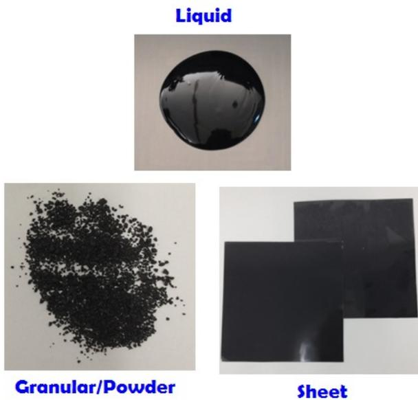
Fig. 7 Different forms of encapsulant.
